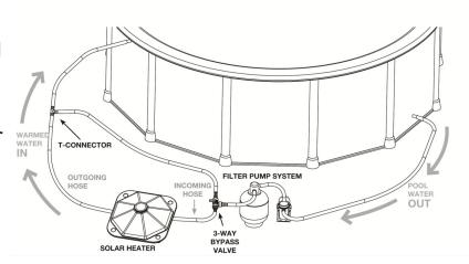
**IMPORTANT NOTE #2:** It is critical that the 3-Way Bypass Valve is **oriented** in the correct way for proper set up. Your pool set up may vary. Refer to page 6 of the instructions for detailed information. Incorrect set up may cause severe damage
